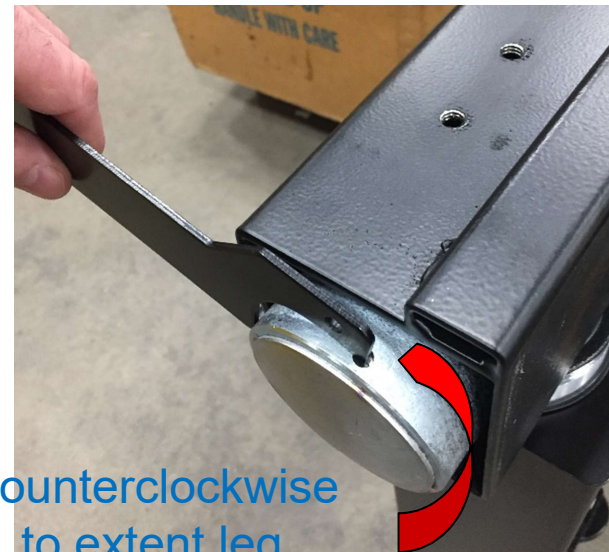
Spanner wrench for leveling feet and caster adjustment 87-17327-00
